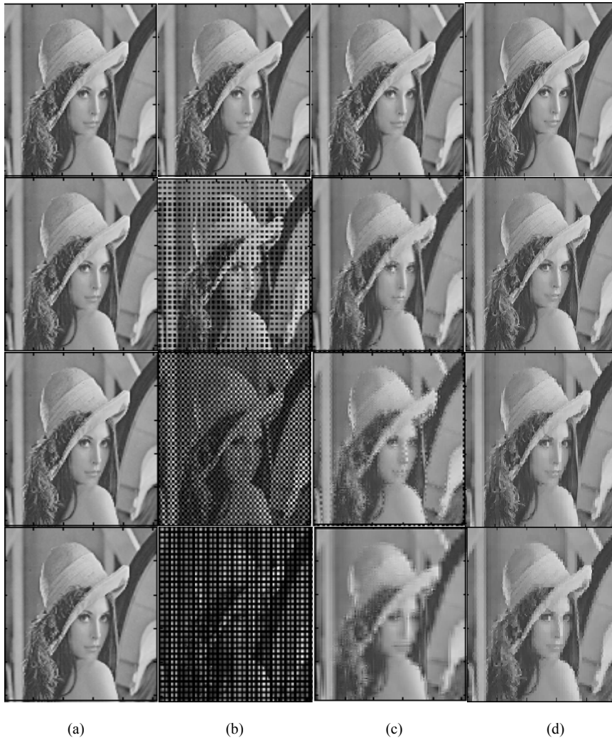
Fig 4 Reconstructed images for 4-channel case: (a) original image, (b) nonhierarchical decomposition without recovery of lost data, (c) nonhierarchical decomposition with mean reconstruction method, and (d) proposed block-based dc coefficient reallocation method. first row - reconstructed images when all (4) channels are available, second row - reconstructed images when 3 channels are available, 3rd row - reconstructed images when 2 channels are available, 4th row - reconstructed images when 1 channel is available.
